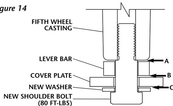
**NORMAL SPACING (A, B & C) AFTER BOLT INSTALLATION.
