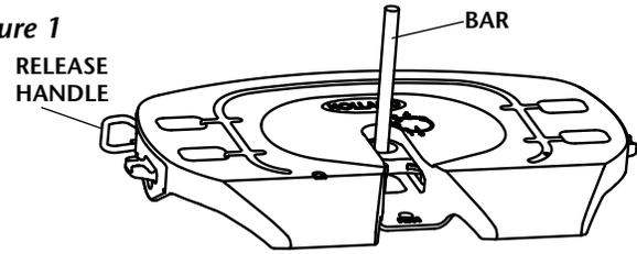
**IMPORTANT:** Use a bar or block to rotate jaw when opening or closing the locking mechanism. When locking the jaw, stand clear of the release handle as it retracts rapidly during lockup.
