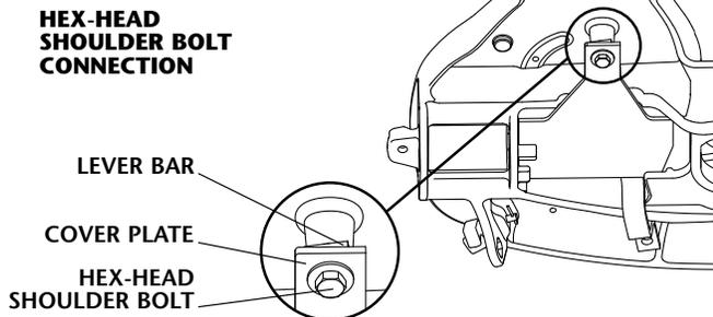
9. Slide the cover plate back until it clears both tabs (Arrow **A**), lift and remove (Arrow **B**) (*Figure 7*).
