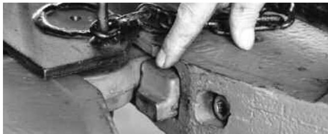
2. Close the locks (using the lock tester), then using a ratchet with a 1/2" Allen wrench, tighten the adjustment screw (*Item 14*) in the throat of the top plate by turning clockwise until tight.
